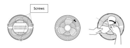
Unscrew the 3 x screws from the back cover and remove the front cover by twisting it to the left.
