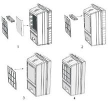
Remove the filter and honey comb from the rear cover for cleaning.
