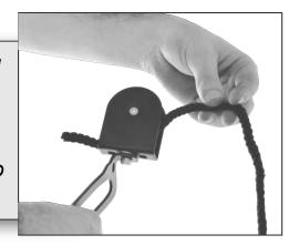
Dress the free end of the Pulley Rope up through the round hole in the bottom of the Pulley Bracket and out the end.
