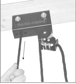
Pull down the rope located between the Pulley Bracket and Hanger. This will pull the knot back into the bracket.
