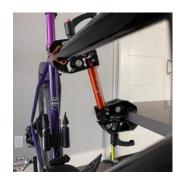
Using the Connect in this configuration is not ideal for carbon bikes as it would mean clamping the top tube (which we DO NOT suggest on carbon) – That said, if it happens to be your only options we have found that simply using the jaw of the clamp as a resting area to suspend your bike up right and in place for basic maintenance such as lubing a chain or airing up your tires is still better than nothing.
