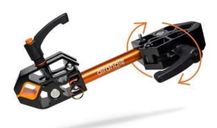
Use the QR Pull Pins (Part 4) to enable the four points of rotation and 2 attachment angles to get the clamp in the best position for the bike and or support structure.
