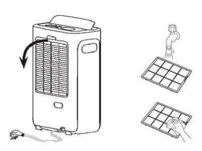
Dust buildup from continuous use can reduce the unit's efficiency. To prevent dust from clogging up the unit, always operate with an air filter in place.
