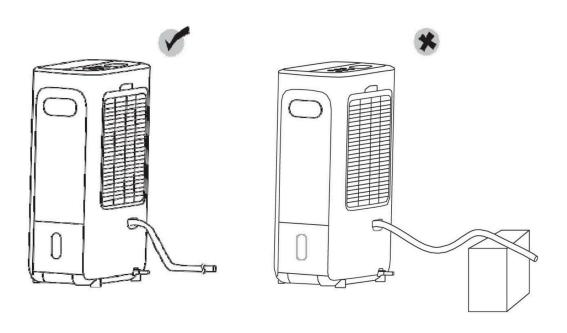
You may use the hose provided or any hose with an inner diameter of 14mm for continuous drainage:
