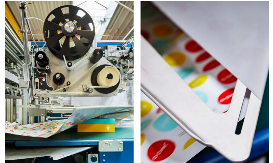
The bag packaging machine uses optical components to detect the size of a product, cuts the required film, welds it to size and prints out the label.
