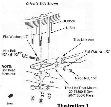
**2)** To install the Trac-Link Rear Mount (20-71800-5 Drvr, 20-71800-6 Pass) support the differential with a floor jack. Unbolt U-bolts and lower rear axle enough to insert the Trac-Link Rear Mount between the lift block and axle housing as shown in **Illustration 1**. Verify that the index pin on the lift block passes through Rear Mount and into the hole in the axle housing. Install U-bolts and tighten assembly.
