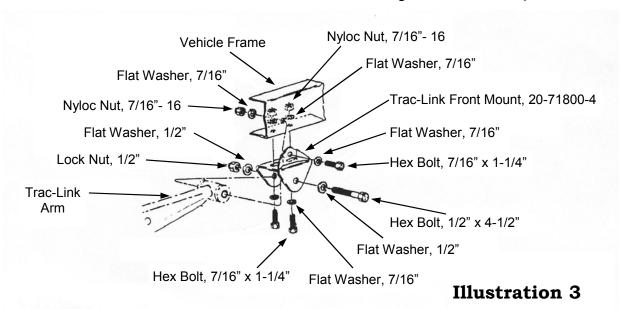
shown in **Illustration 3** and tighten assembly. Tighten 1/2" Link-to-Mount bolts once vehicle is at ride height.
