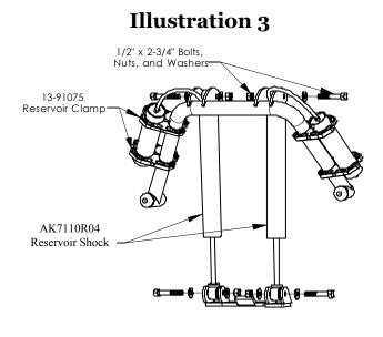
RCD Suspension 619-588-4723 Page 5 - #16-32305 **NOTE:** If using reservoir shocks, install shocks with hoses facing outward and clamp reservoirs to hoop on the outside of the tube. Be sure to check mounting position of reservoirs, clamps, and hoses as to not interfere with wheel and tire assembly.
