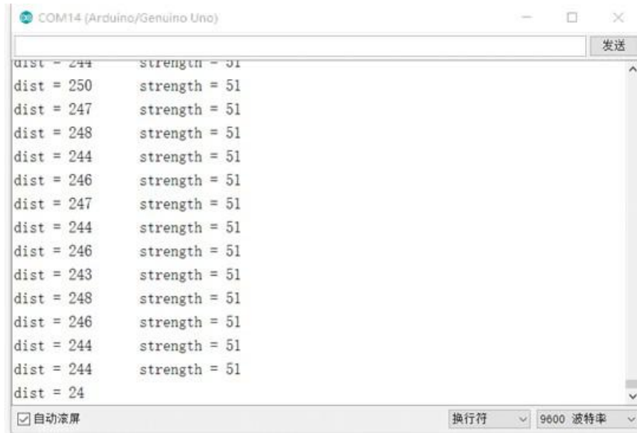
Figure 3 Display of LiDAR's Data on Monitor for Serial Port
