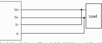
Note: 1. The left side represents the internal schematic diagram of the product, the right side represents the customer system; 2. Twisted pair wires are needed for S+/S-.
