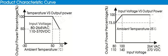
Note: 1. With an AC input voltage between 80-100VAC and a DC input between 110-140VDC the output power must be derated as per the temperature derating curves;
