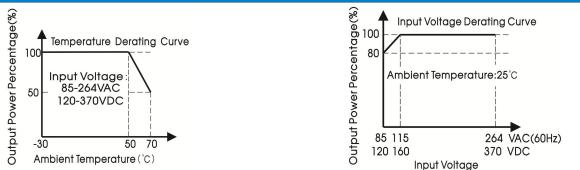
Note: 1. With an AC input voltage between 85-115VAC and a DC input between 120-160VDC the output power must be derated as per the temperature derating curves;
