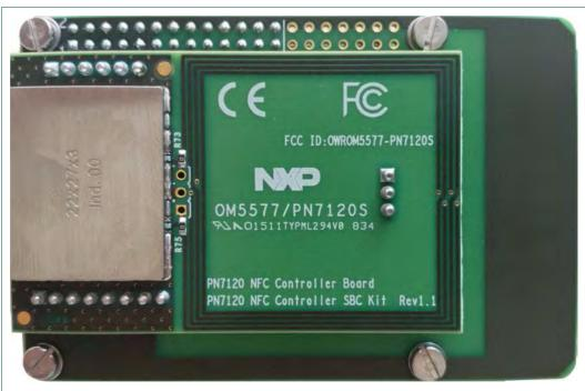
Fig 2. OM5577/PN7120S Raspberry Pi configuration
