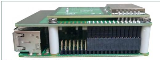
Fig 4. OM5577/PN7120S and Raspberry Pi B+ model stacked together
