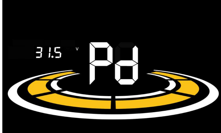
Figure 6-13 Battery under voltage value setting interface
