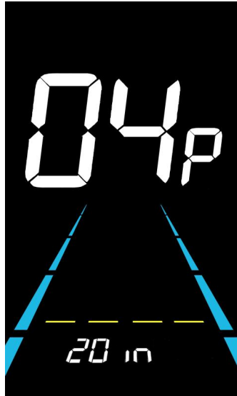
Figure 6-5 Wheel diameter setting interface
