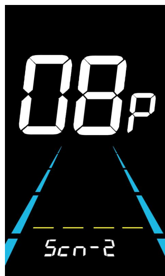
Figure 6-10 PAS sensor sensitivity setting interface
