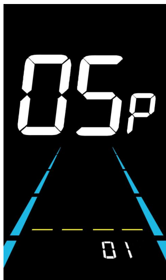
Figure 6-6 Number of speed sensor magnets setting interface
