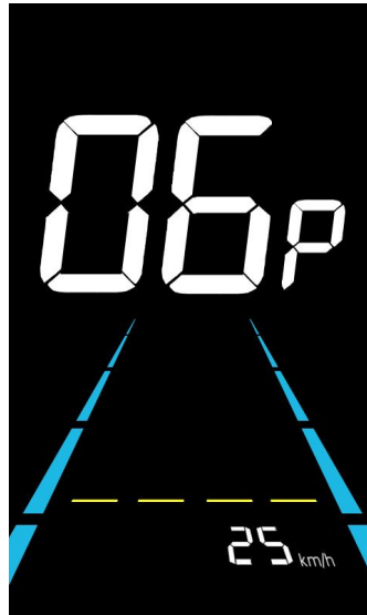
Figure 6-7 Speed limit setting interface
