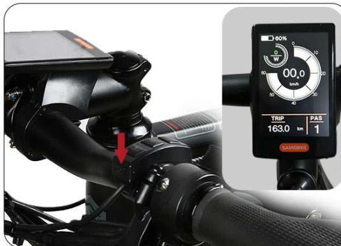
Then press the instrument power key to start the ebike system
