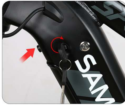
Turn the key clockwise to unlock the battery lock, then press the button.
