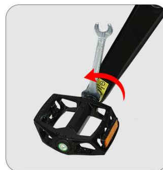
Tighten the left pedal "L" counterclockwise
