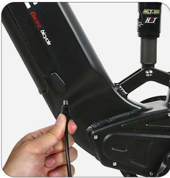
Plug the charger into the power hole
