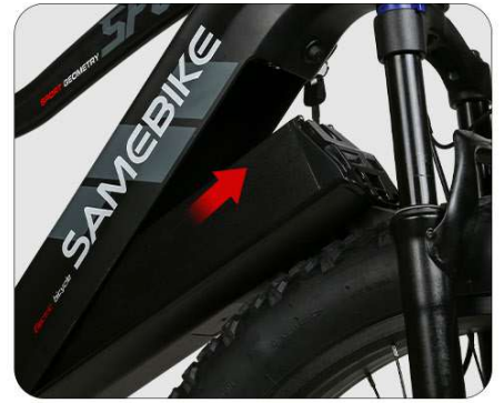
Remove the battery upwards
