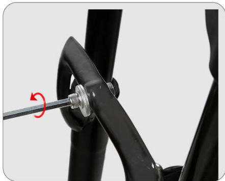
Loosen the set screw counterclockwise
