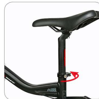
Adjust the proper height and lock the clamp
