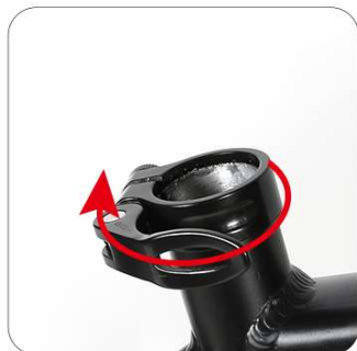
Open the clamp in the direction of the arrow
