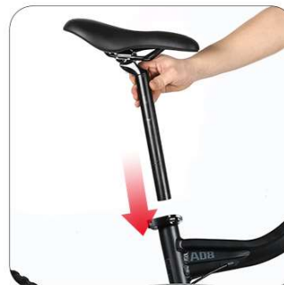
Insert the saddle into the seat tube
