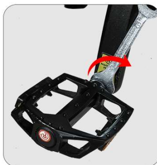
Tighten the right pedal "R" clockwise
