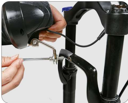
Put in and tighten the headlights and front fender respectively
