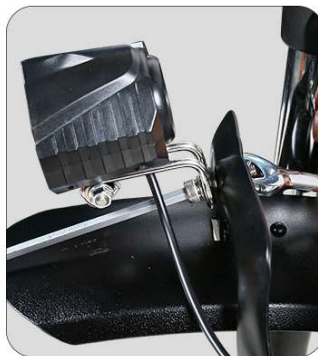
Install the headlights and front fender
