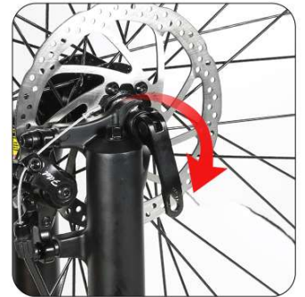
Lock the quick release handle to complete the front wheel installation
