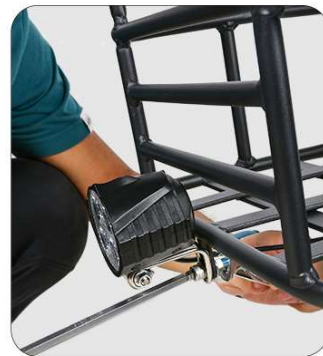
Finally, headlights can be installed under the basket
