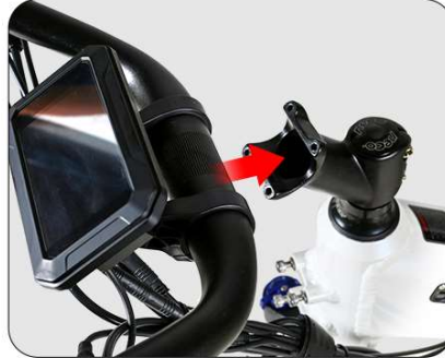
Install the handlebar to adjust the direction
