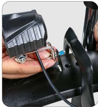
Put in and tighten the headlights and front fender respectively
