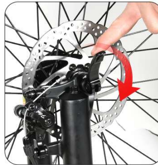
After screwing to a certain strength, fasten the quick release handle in the direction of the arrow
