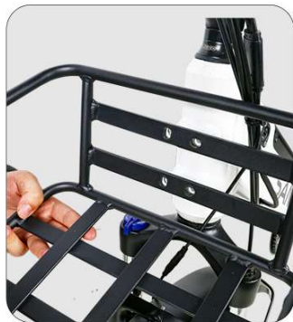
Loosen the head screws, align the basket screw holes with the head screw holes
