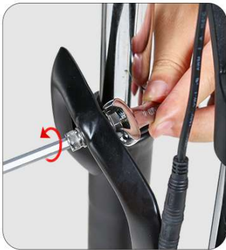
Loosen the set screw counterclockwise
