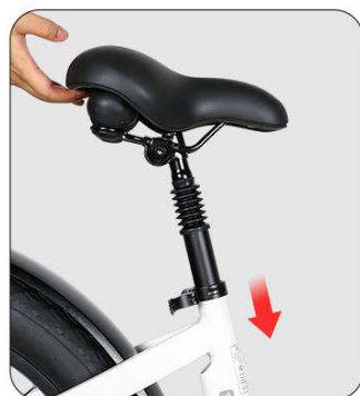
Insert the seat tube in the direction
