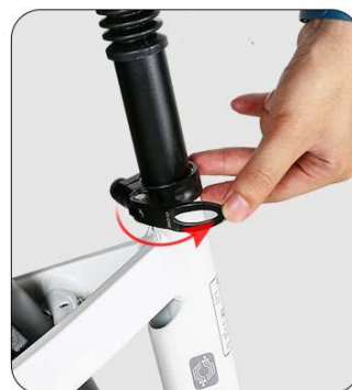
After adjusting the seat direction and height, lock the quick release lever
