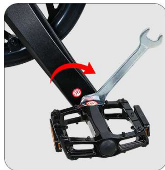
Tighten the right pedal "R" clockwise
