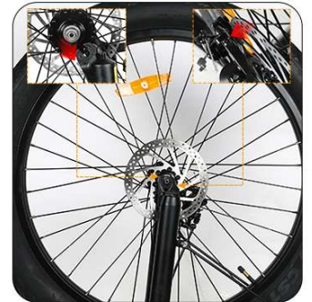
Install the side with the ebiked disc into the direction with the disc brake
