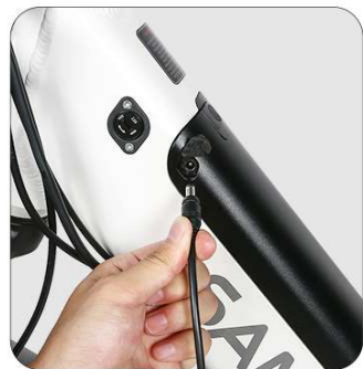
Plug the charger into the power hole
