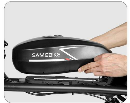
Remove the battery
