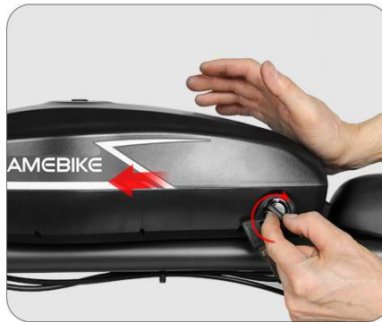
Turn the key clockwise to unlock the battery lock, then push it forward
