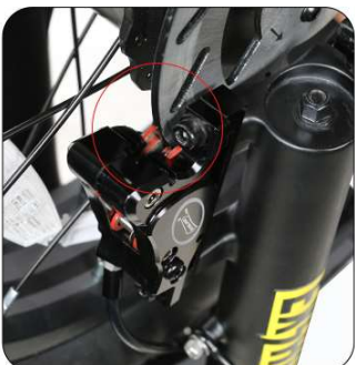
Install the side with the ebike disc into the direction with the disc brake
