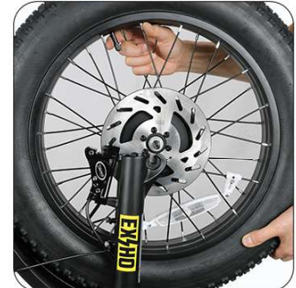
Put the tire into the fork
