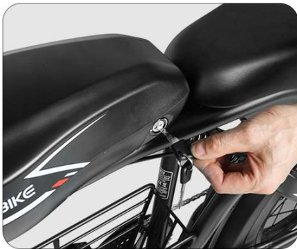
Shut down the power
