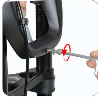
Loosen the front fork screws with a hexagonal screwdriver
