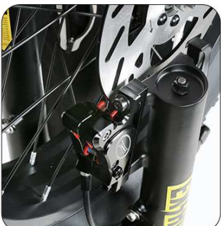
Install the side with the ebike disc into the direction with the disc brake
