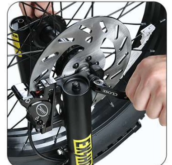
After screwing to a certain strength, fasten the quick release handle in the direction of the arrow
