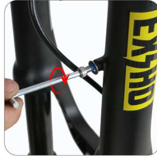
Loosen the screws on both sides of the front fork
