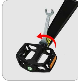
Tighten the left pedal "L" counter clockwise
