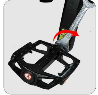
Tighten the right pedal "R" clockwise
