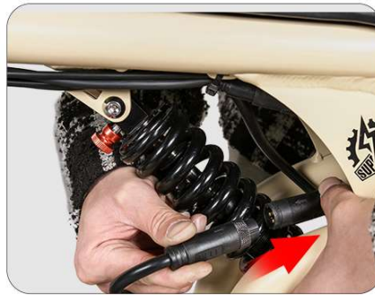
Rotate the plug so that the arrow on the plug is aligned, then connect the plug
