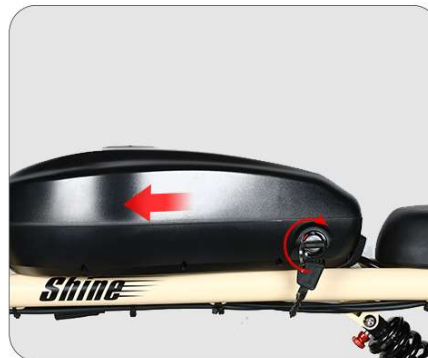
Turn the key clockwise to unlock the battery lock, then push it forward
