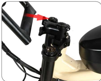
Install the handlebar to adjust the direction
