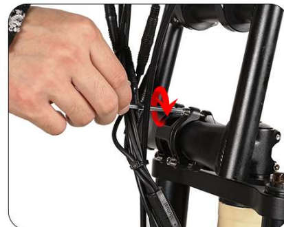
Tighten 4 screws to fix the handlebar
