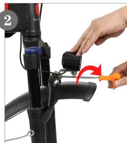
2 Put the headlights and the front fender into the screws and tighten them
