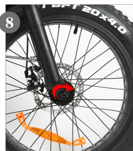
8 Tighten the quick release part in the direction
