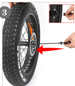
3 Insert the quick release handle into the rim shaft hole
