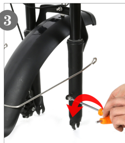
3 Loosen the screws on both sides of the front fork
