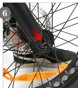
6 Put the opposite side of the disc brake pads into the opposite side of the brake disc
