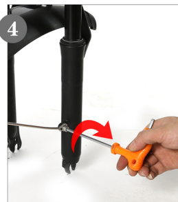
4 Tighten the brackets on both sides of the front fender
