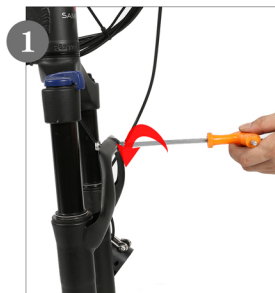
1 Loosen the front fork screws with a hexagonal screwdriver
