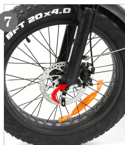
7 Tighten the quick release handle in a clockwise direction
