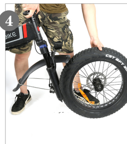
4 Put the tire with quick release handle into the front wheel
