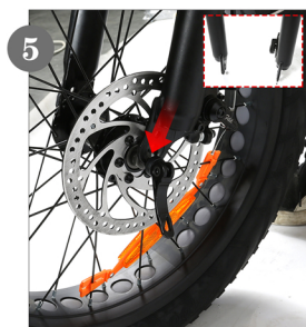
5 Put the brake disc on the side where the disc brake is installed
