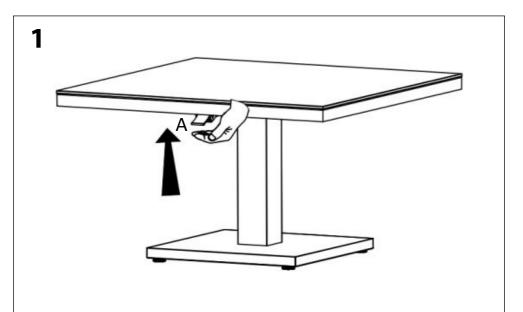
Press handle **A.** The table top will go up automatically. You can stop the table at any desired height.
