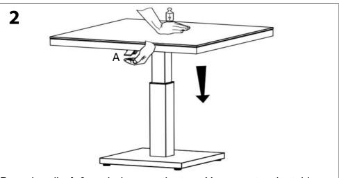
Press handle **A** & push down on the top. You can stop the table at any desired height.
