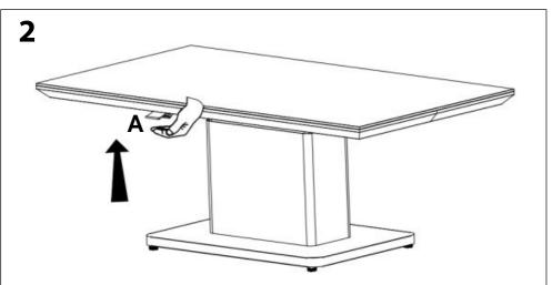
Press handle **A.** The table top will go up automatically. You can stop the table at any desired height.
