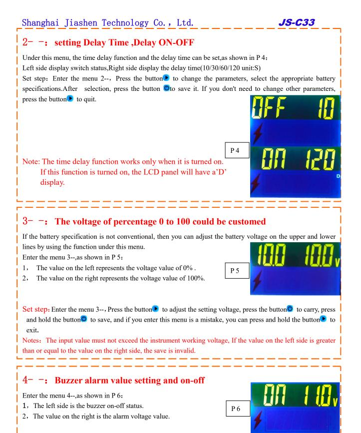
Set step: Enter the menu 4--, press the button ●to take the buzzer on or off, press the button<sup>(1)</sup> to carry, press and hold the button<sup>(2)</sup> to save, and if you enter this menu is a mistake, you can press and hold the button<sup>(1)</sup> to exit.
