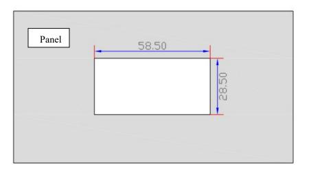
Notes: panel thickness 2-3MM best, Please adjust the slotting size according to the panel material
