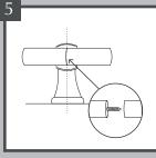
A double ended screw is provided to connect to two pole parts, the central bracket will cover the join. The cut ends will have to be re drilled to fix the finials, please use the template provided to ensure the drill hole is central.
