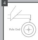
Cut the pole to the overall length required remembering to include the length of the finials in your calculation. If you need to cut the length of a two piece pole set you need to cut equal amounts off each pole at the finial end.
