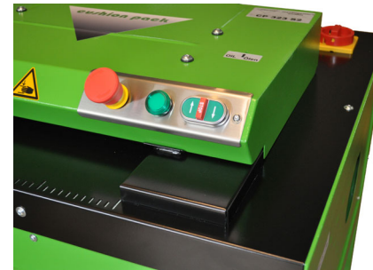
controls and circuit-breaker according to IEC/EN 60204-1
