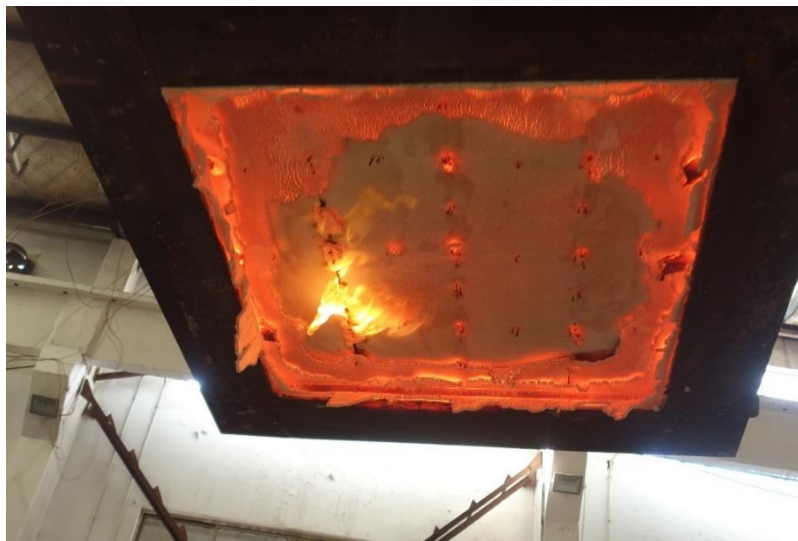
Photo No. 14 Exposed Surface after Fire Endurance Test (120 minutes)
