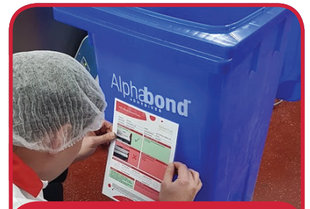
Image 8: A lidded bin for storing the adhesive will stop debris entering the adhesive which then blocks nozzles.
