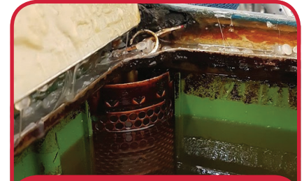
Image 11: Early generation adhesive went dark in the tank through charring and oxidation.
