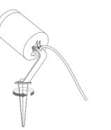
Install each spotlight on the ground and adjust the angle of its beam.
