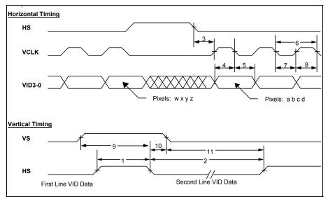
Figure 2. Video Input Timing Diagram.
