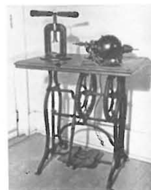
Lathe and press for swedging dentures and old electric motor equipped with brush for polishing plates and teeth.
