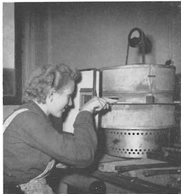
The ovens in which the teeth are baked are carefully watched and timed, and the finished products are considered to be among the finest teeth in the world.
