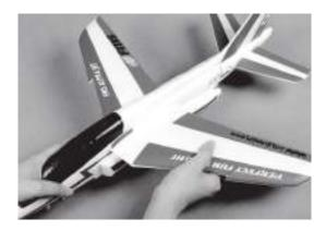
2.Make sure that the horizontal stabilizer is symmetrical and aligned with the fuselage(body) of your Alpha jet.
