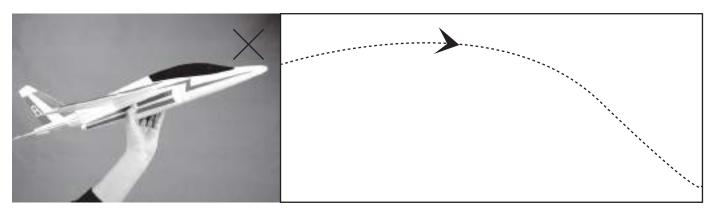
2.Damage to the nose of the Alpha jet may occur if the nose is pointed down at an angle greater than 10 degrees.
