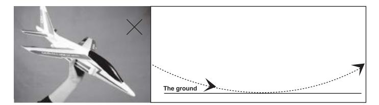
3.To achieve optimun flight results ,throw your Alpha jet at an angle between plus and minus 10 degrees. The Alpha jet should follow the trajectory as shown on the diagram below.
