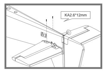
2.Install the servo arms and linkage rods as shown.
