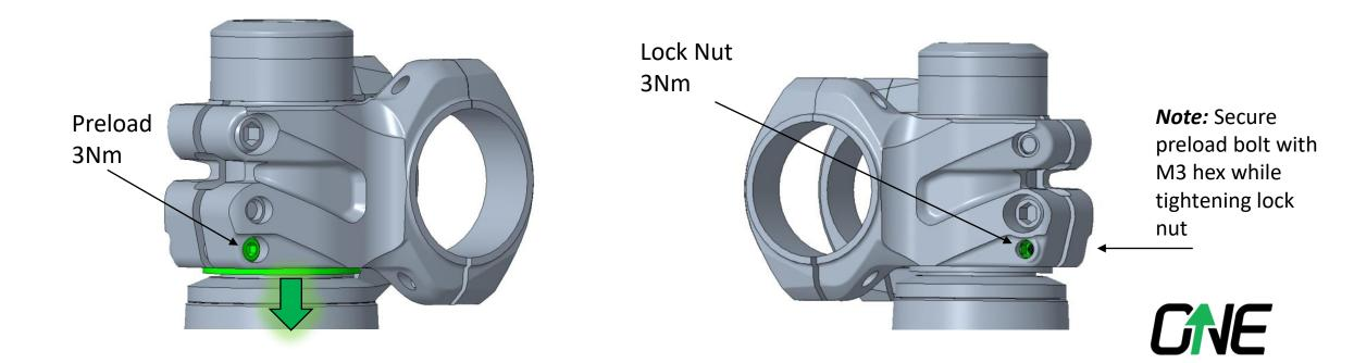
10) If the headset is tight then lock the preloader. Secure the preload bolt using an M3 hex and tighten the lock nut on the left of the stem using an M4 hex to 3Nm.
