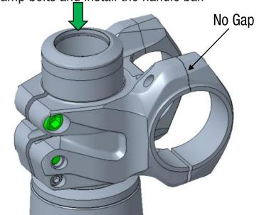
Tighten the top bar clamp bolts first, there will be no gap between the bar clamp and stem. Bottom bolts will have a gap between the clamps and stem body after tightening. Torque to 6Nm.
