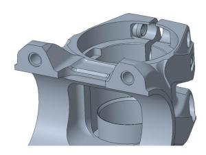
2) Install the preload collar into the stem. With the upside-down stem in your hand take the collar (which has neither nut or bolt in it) make sure the cone shape is opening outward and angle the closure of the collar into the stem. Then insert a 4mm hex wrench in from the right to pinch the closure slightly. This will allow the collar to seat into the stem
