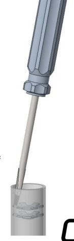
1) With the Stem upside down, install the headset preload lock nut into the stem. Do this by dropping it in from the right. It must be oriented this way and will be on the left side once in place.
