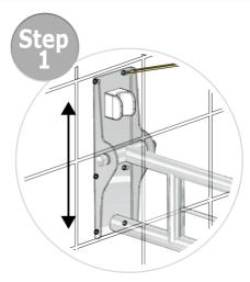
Assemble the rail intoposition.
