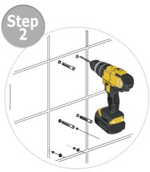
(2) Drill the holes with a suitable wall/tile drill piece. Use masking tape to mark the wall and drill through, protecting the tile from splintering.
