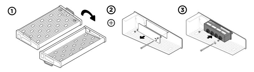
The 4X MOD mounts in the Modular Endpanel of your Templeboard and allows you to route  $\frac{1}{4}$ " inputs and outputs through the side of your board.
