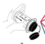
Remove filter cap, push plunger to eject used coffee and rinse seal.
