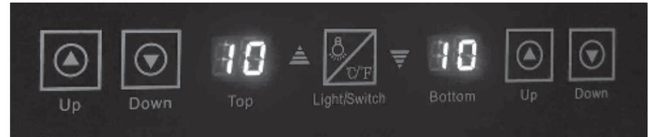
2. Set the desired cooling temperature by pressing the buttons ▲ or ▼ to set your desired temperature. Each depression of the buttons will scroll through the available temperature settings. Numbers will flash while setting. Solid numbers indicate the current internal temperature in Celcius degrees.
