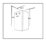
Allow sufficient clearance to insure proper air circulation: 30 cm (12") at the top and 10 cm (4") on each sides and back of the unit.
