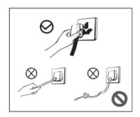
Do not pull the cord when trying to disconnect the freezer. Firmly grasp the plug and pull out it from the socket directly.
