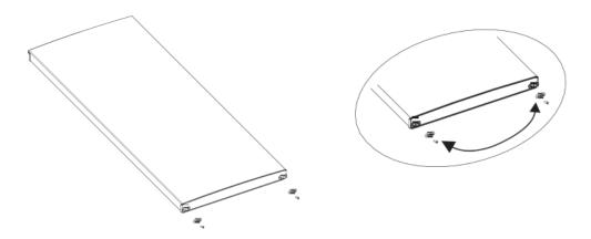
5) Dismantle the lower hinge and adjustable leg;
