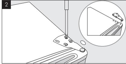
Using a slotted screwdriver, unscrew the three screws from the top hinge bracket. Remove the bracket. Lift and remove the door from the bottom hinge pin. Set door safely aside.
