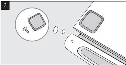
On the opposite side of the unit, use a thin-bladed tool to carefully pry up and remove the hole plug from top of door and plastic square cover from top of cabinet. Insert plug and cover into provided hole on opposite side of door and into holes exposed by removal of top hinge bracket.
