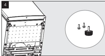
Unscrew and remove the leveling foot from the bottom hinge bracket. Using a slotted screwdriver, remove the two screws attaching the bottom hinge bracket to the cabinet. Unscrew the foot from the other side of cabinet. Attach bracket and feet to opposite sides from which removed.
