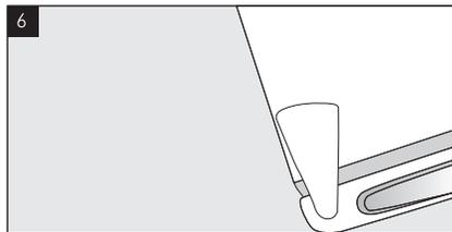
Replace the plastic hinge cover over the top hinge bracket.
