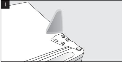
Using a flat blade screwdriver, remove the plastic hinge cover from the top of door. Be careful not to scratch refrigerator surface.
