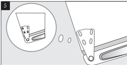
Mount the door onto the bottom bracket. Insert the top bracket hinge pin into the hole on top of the door. Use the three previously removed screws to attach back of the top bracket to cabinet.
