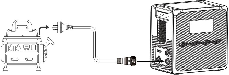
**Note:** Make sure your generator delivers the AC output with charging voltage, frequency, and Grid Self-adaption Mode voltage that meet AC240's specifications.
