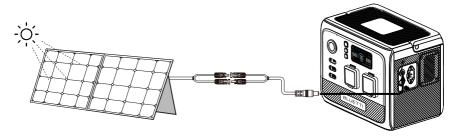
Warning: The open circuit voltage of solar panels cannot exceed 28V, otherwise it will damage the device. (Note: This is not covered in the warranty.)
