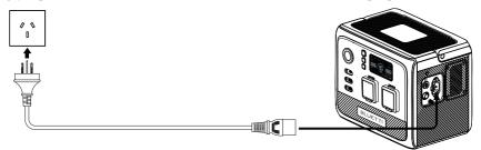
AC60 supports Turbo/Standard/Silent charging modes. It's set to standard charging by default, while the Turbo and silent modes can be enabled in BLUETTI app. BLUETTI's AC charging mode guide is as follows:
