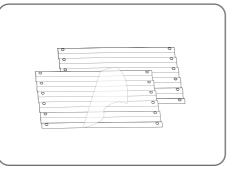
Remove the protective film from both sides of the panels prior to assembly Step 2
