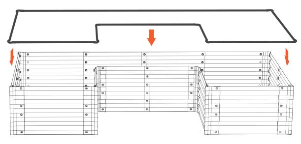
(You can use the back of the wrench we provide or a screwdriver to slightly open the channel of the rubber edging only at the joints where the panels overlap allowing it to slip over both panels easier.)
