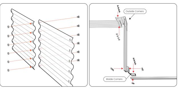
After you have loosely assembled your desired shape, add the interior bolts on the outside and the washer and nut on the inside
