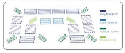
Lay out the Corners and Panels in the design you wish to build. Make sure the inside ( ) and outside ( ) corners are layed out correctly.
