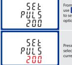
From the set-up menu, use MD and P buttons to select the Pulse width option.
