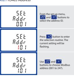
On completion of the entry procedure, press button to confirm the setting and press Win button to return the mair
