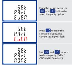
On completion of the entry procedure, press to confirm the setting and press to return to the main set up menu.
