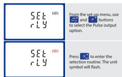
On completion of the entry procedure, press to confirm the setting and press to return to the main set up menu.
