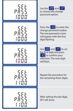
Press WA to exit the number setting routine and return to the Set-up menu. SET will be removed
