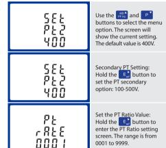
The PT Rate is the PT Primary divided by the PT Secondary. For Example: Voltage Transformer -  $11000\div110=100$ , so the PT Rate would be 0100 and the PT2 would be 110.
