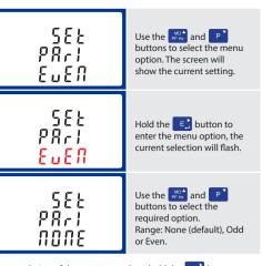
On completion of the entry procedure, hold the Et button for 3 seconds until the selection stops flashing.
