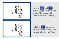
Use the provide and provide buttons to choose the desired pulse rate. To save the new setting, hold the c, button for 3 seconds until the selection stops flashing.
