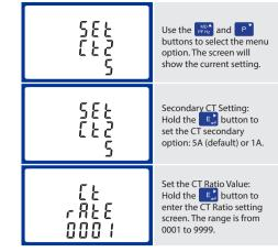
Example: 200/5A Current Transformers - 200÷5=40, so the CT Rate would be 0040 and the CT2 would be 5. On the MID Version, you can only program the CT Rate ONCE.
