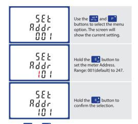
Use the end and buttons to choose the necessary number, then press the button to move along to the next number. To save the new setting, hold the button for 3 seconds until the selection stops flashing
