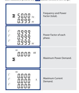
Each successive press of the P button select a new range: 0.000 \*\*\* 0.000 L  $L^2$ Instantaneous Active Power in kW. L<sup>3</sup> 0.000
