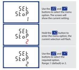
On completion of the entry procedure, hold the for 3 seconds until the selection stops flashing.
