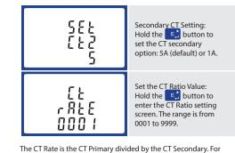
Example: 200/5A Current Transformers - 200 $\div$ 5=40, so the CT Rate would be 0040 and the CT2 would be 5.
