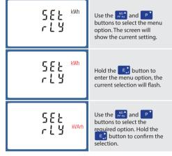
Hold the VA button for 3 seconds to exit the set up menu.
