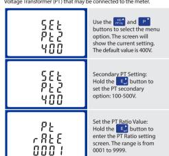
The PT Rate is the PT Primary divided by the PT Secondary. For Example: Voltage Transformer - 11000÷110=100, so the PT Rate
