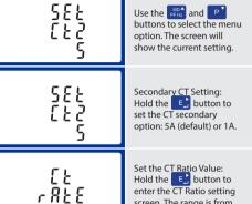
The CT Rate is the CT Primary divided by the CT Secondary. For Example: 200/5A Current Transformers - 200÷5=40, so the CT Rate would be 0040 and the CT2 would be 5.
