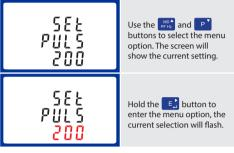
Use the Price and P buttons to choose the desired pulse rate. To save the new setting, hold the button for 3 seconds until the selection stops flashing.
