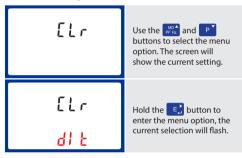
Hold the button to confirm the setting and press MA to return to the main set up menu.
