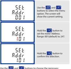
Use the P buttons to choose the necessary number, then press the button to move along to the next number. To save the new setting, hold the button for 3 seconds until the selection stops flashing
