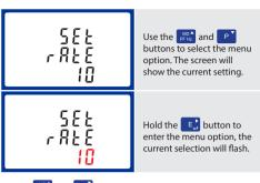
Use the P buttons to choose the desired pulse rate. To save the new setting, hold the button for 3 seconds until the selection stops flashing
