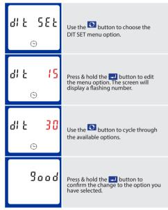
To exit the set-up menu, press & hold 💽 until the measurement screen is restored.
