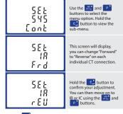
Hold the WA button for 3 seconds to exit the set up menu.
