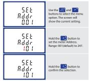
Use the and p buttons to choose the necessary number, then press the button to move along to the next number. To save the new setting, hold the button for 3 seconds until the selection stops flashing.
