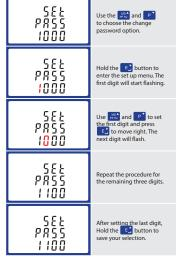
Hold the WA button for 3 seconds to exit the set up menu.
