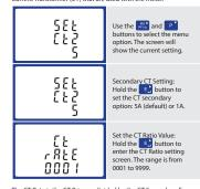
The CT Rate is the CT Primary divided by the CT Secondary. For Example: 200/5A Current Transformers - 200+5=40, so the CT Rate would be 0040 and the CT2 would be 5.
