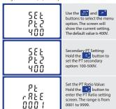
The PT Rate is the PT Primary divided by the PT Secondary. For Example: Voltage Transformer - 11000+110=100, so the PT Rate would be 0100 and the PT2 would be 110.
