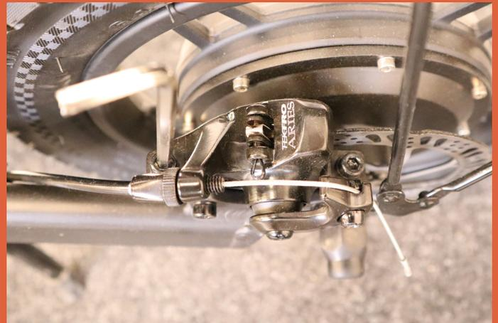
3. Adjust the static brake pad so that it aligns with the metal corner of the caliper
