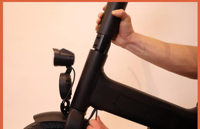
5. Feed the brake wire into the frame.
