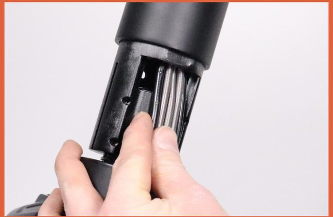
3. Pull brake cables out, be careful not to damage wire housing
