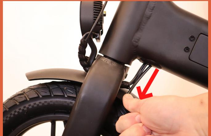
4. Now mount the steering pole while carefully pulling the brake wire
